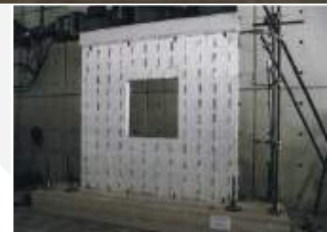
Left: Seismic test on ISOTEX two-storey wall Above: Seismic test on full ISOTEX wall Rights: Seismic test on ISOTEX wall with window
