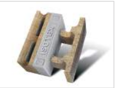
Isotex Air ventilate block HDIII 44/11 with Neopor® BMBcert by BASF - U=0,19 W/m²K
